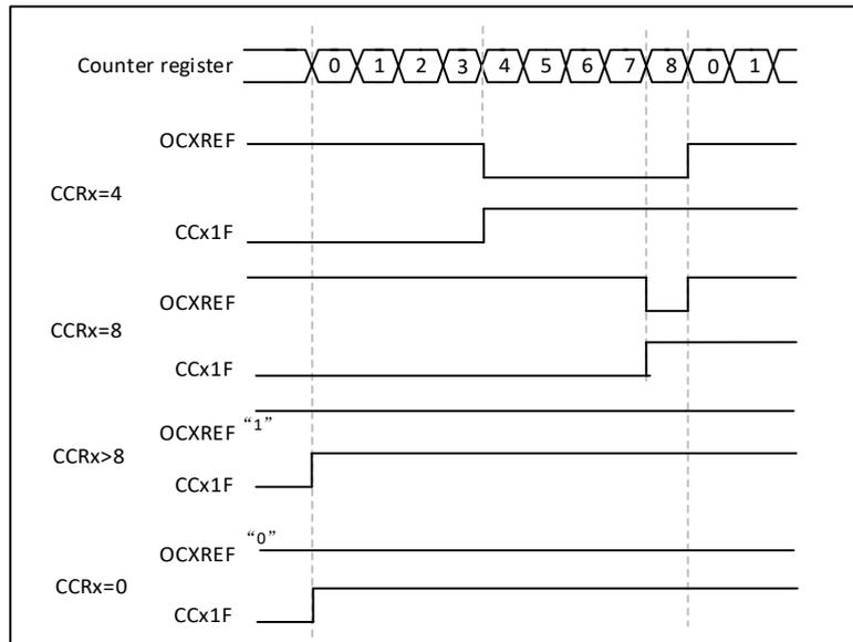
图 21-29 Edge-aligned PWM waveforms (ARR=8)
