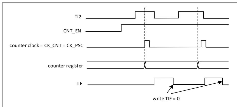
图 21-23 Control circuit in external clock mode 1
