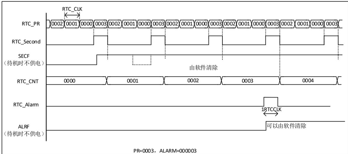
图 28-2 RTC 秒和闹钟波形图示例, PR=0003, ALR=00003
